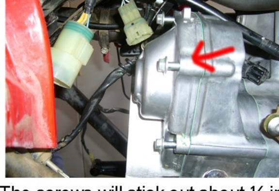
Grease the seal and install the alternator case Note: the magnets will make the case difficult to install
