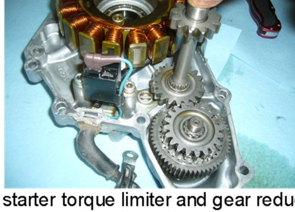
Install the starter torque limiter and gear reduction shaft in the alternator case
