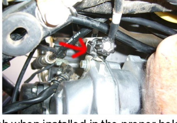
Grease the seal and install the alternator case Note: the magnets will make the case difficult to install
