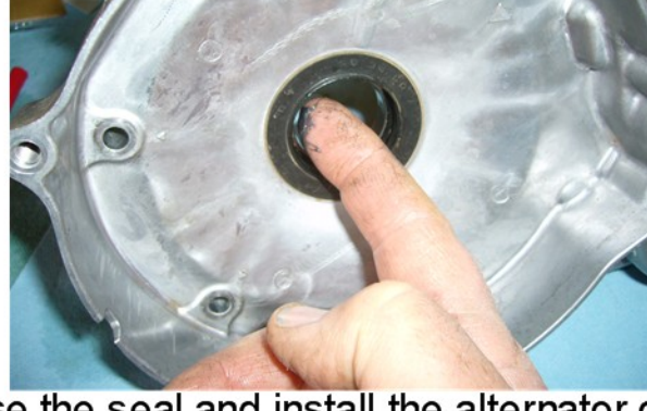
Grease the seal and install the alternator case Note: the magnets will make the case difficult to install
